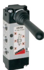
G1/8", 5/3 CO Lever Valve Bistable
