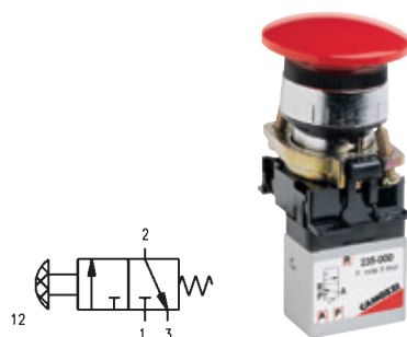
3/2 Palm Switch Spring Return Valves
