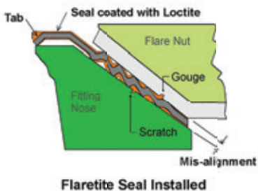
Flaretube Seal Installed
