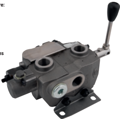
3/4" BSPP, 1406 Series, 3 Position, Single Section, Open Centre, 85-175 bar Relief Valve
